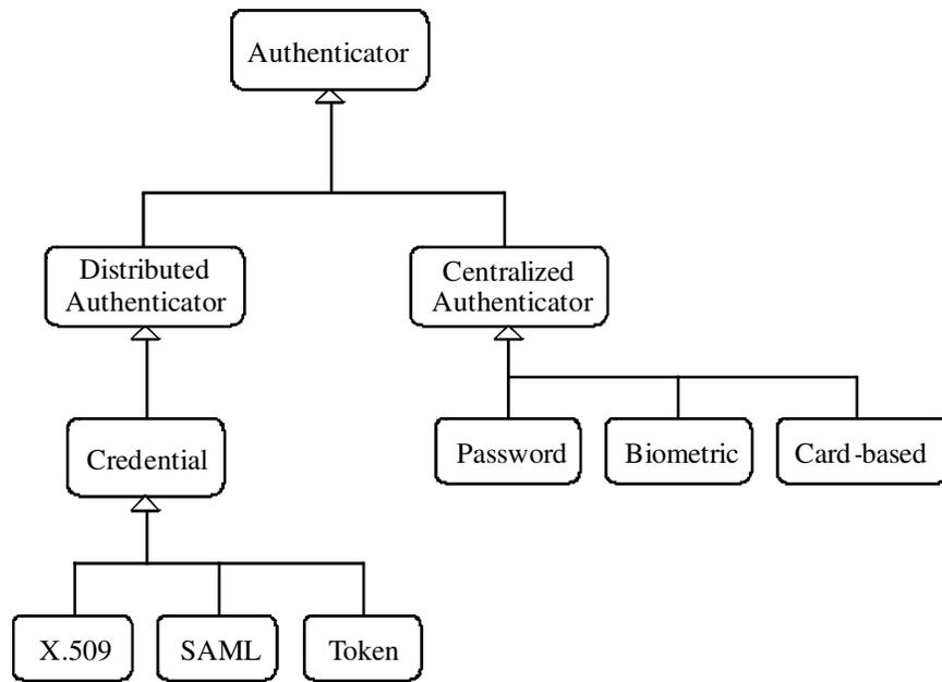
**Fig. 3.** Pattern diagram for the authentication hierarchy
