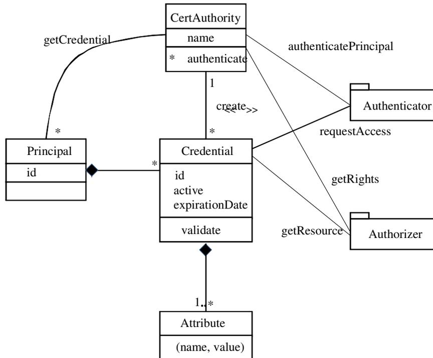
**Fig. 2.** Class diagram of the Credential pattern (from [7])
