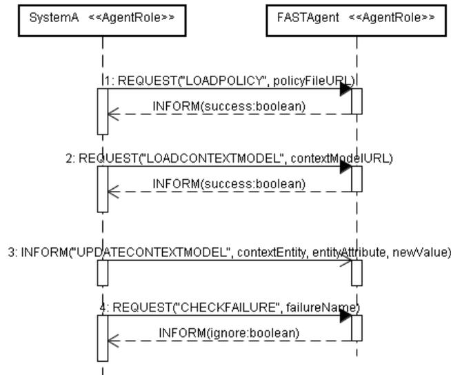
**Fig. 4.** Communication between a system and the FAST Agent
