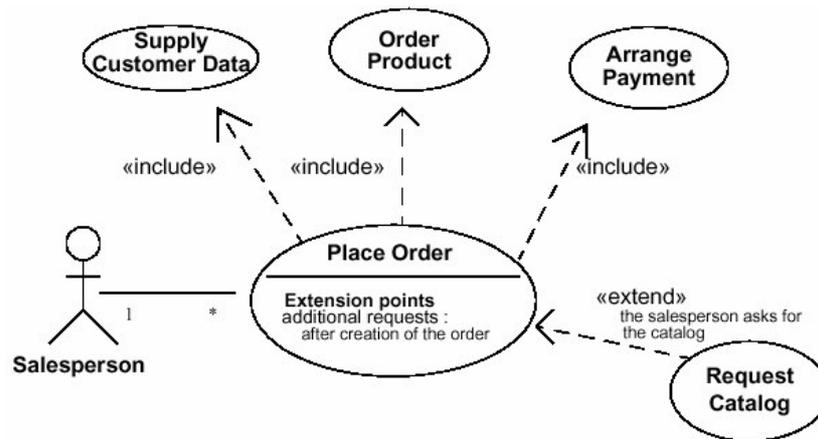
Figure 1. A use case diagram extracted from the UML Specification v1.5, pp.3-99 [4].
