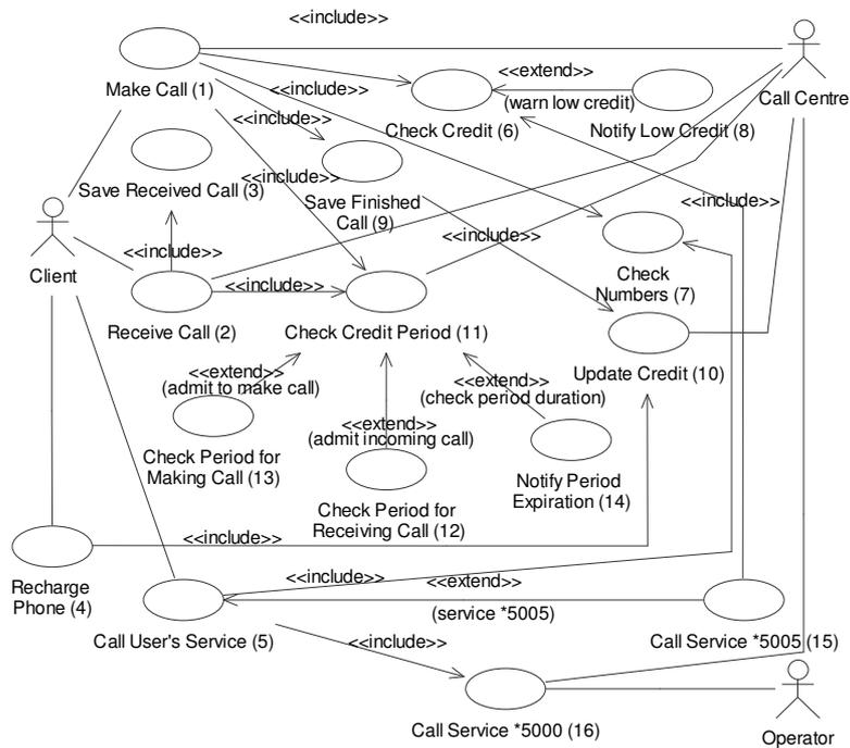
Figure 2. Use case diagram of a system for monitoring and billing cell phone calls (billing system). The number at the end of each use case's name is its identifier.
