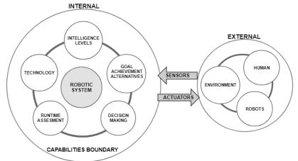
Fig. 2. Requirement abstraction for robotic system.
