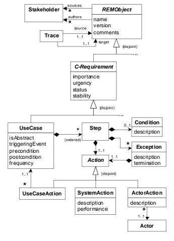
Figure4. UML model of use cases in REM
